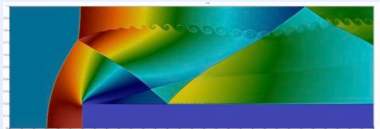
Supersonic compressible Euler flow past a forward facing step; notice the beautiful ripple of the horizontal slip-line. This Active Flux simulation is from Duan, Barsukow, Klingenberg, SAM Journal on Scientific Computing, vol. 47, no. 2 (2025)
