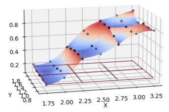
Here we see six rectangular computational cells (violet). In each cell the solution of a PDE is reconstructed to third order (the blue and red surface) using the information given by the black dots. These six surfaces together give a continuous reconstruction.
