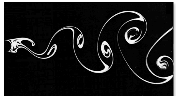
flow past a cylinder, the so called von Karman vortex street
