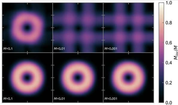
An analytic solution (the Gresho vortex) is numerically computed for various Mach numbers ( $10^{-1}, 10^{-2}, 10^{-3}$ ). The picture of the analytic solutions looks the same in all these cases. The bottom row is our scheme, the top row is not.
