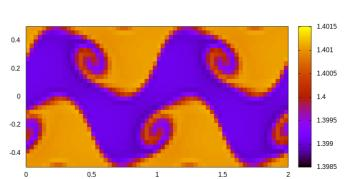
In this simulation a shear flow causing the roll up of vortices is seen. The simulation on the left is done on a coarse grid, but still the vortex is resolved extremely well.
