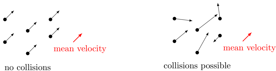
Figure 2.7: In both illustrations, the fluid’s mean velocity is the same. In the left illustration, each particle’s velocity coincides with the mean velocity so that the relative velocities vanish. Collisions between particles are not possible. However, in the right illustration, all particles have different velocities (in direction and absolute value) which results in very distinct relative velocities. This can lead to collisions.
